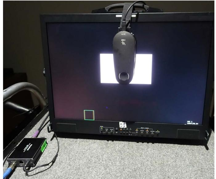
Calibrating takes about 5 minutes. Using a laptop and the probe, the monitor is cycled through a series of color patches. Position probe on monitor. Run IS-Mini Manager Software on laptop.
